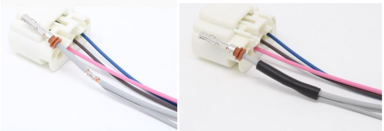
Photos 3A and 3B. The VaporWorx 20ga grey wire is tied into the FSCM fuel pump+ wire. Use a small amount of solder to make the connection and seal with heat shrink or rubber self-sealing tape.
